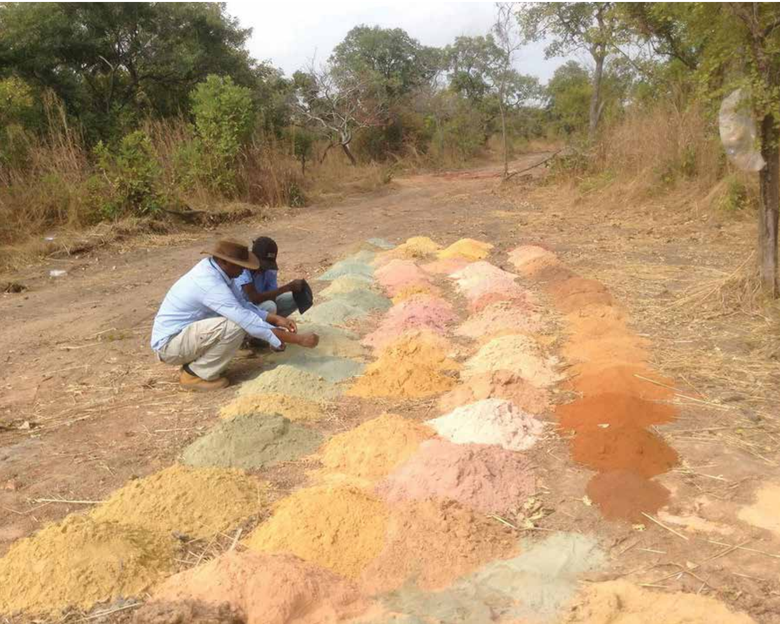
RC drilling chip piles
